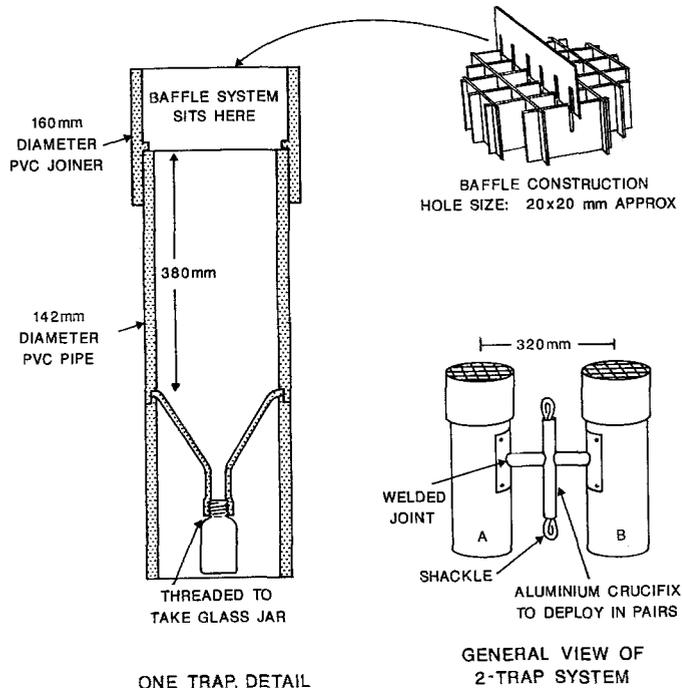
Fig. 2. Design of sediment traps deployed in Davies Reef lagoon
